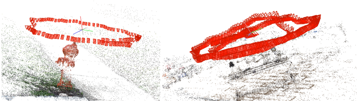
Figure: The above image showcases a point cloud and camera poses for each frame used to create that map using COLMAP of a Fire Hydrant and a Table with an object on it.
